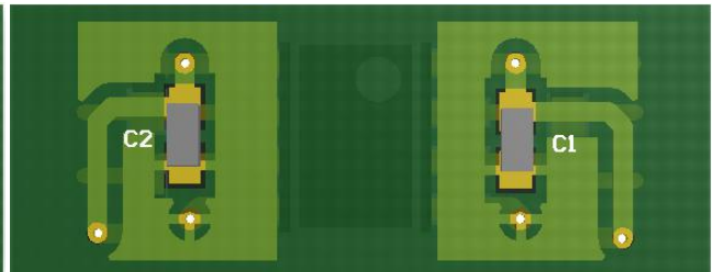
Figure8.2 Recommended PCB Layout — Bottom Layer
